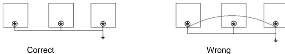
Figure 3-6 Connection of conduction and radiation interference solutions
